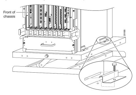
Step 6 With one person positioned on the side of the router to prevent it from tipping, use the 3/4-inch (19-mm) socket and ratchet wrench to turn the scissor-jack screw clockwise slowly and close the scissor-jack platform to lower the chassis. (See Figure A-6.)
